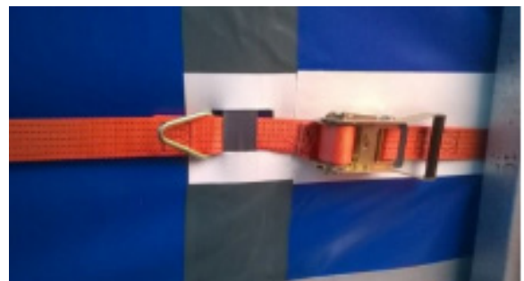
Securing Ring has travelled too far past the white marker
